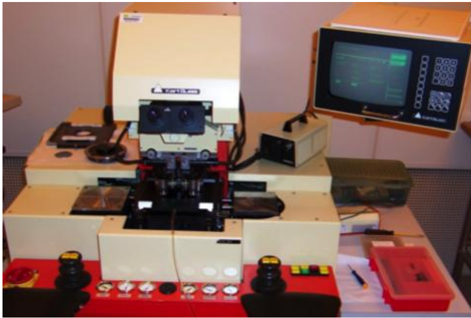
Figure 3.1: (a) The resist-coated wafer exposure setup under a UV light. (b) The primary tool used for emitting UV radiation. (The image is from Nanotechnology Research & Education Center of University of South Florida.
