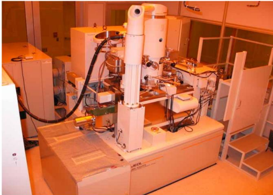
Figure 3.5: JEOL JBX-9300FS electron beam lithography system. (Courtesy Georgia Institute of Technology Nanotechnology Research Center (TNRC))
