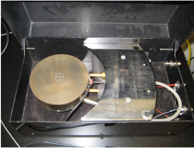
Figure 51. Modified chuck of Signatone system to allow liquid nitrogen to be used as a coolant.
