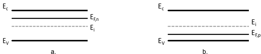
Figure 13 Fermi level at equilibrium in a) n-type and b) p-type semiconductor. E_c and E_v are conduction and valence band edges, respectively.
