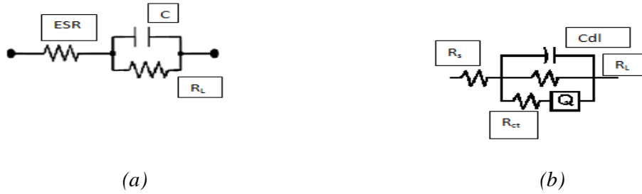
Figure 8: (a) Randle's circuit model, (b) Randle's circuit model with constant phase element
