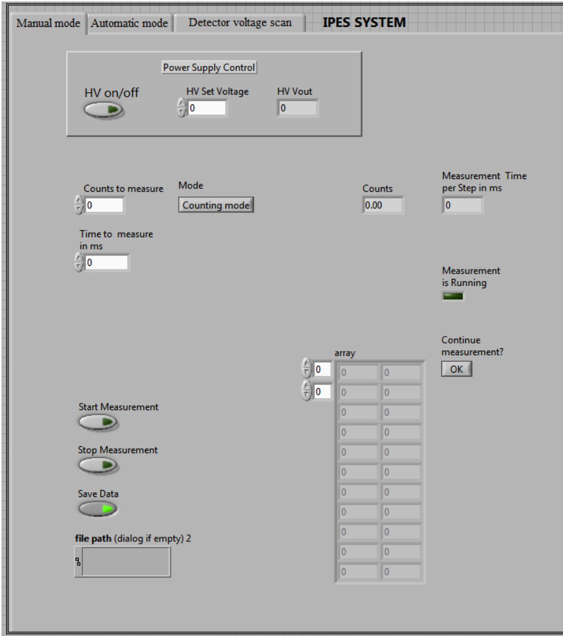
Figure 15: Manual mode for IPES measurement at a fixed electron energy.
