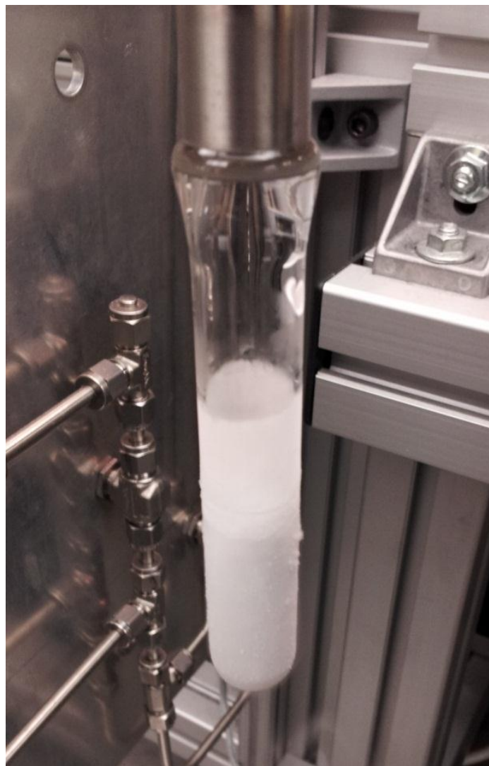
Figure 20: Frozen acetone while evacuating the vial.
