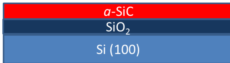
Figure 2.6: Cross-section showing the structure of type II a -SiC developed for testing in this research. The a -SiC was \sim 300 nm thick, deposited on 800 nm thick SiO 2 and deposited on 500 \mu\text{m} thick Si (100) substrate.
