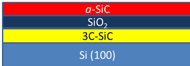
Figure 2.8: Cross-section showing the structure of type IV a -SiC developed for testing in this research. The a -SiC was \sim 300 nm thick, deposited on 800 nm SiO 2 , deposited on \sim 6.2 \mu\text{m} 3C-SiC and grown on 500 \mu\text{m} thick Si (100) substrate.
