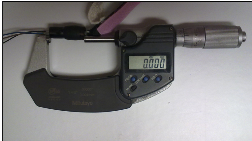
FIGURE 2.11: Respiratory sensor with no displacement measured by the micrometer. The micrometer is calibrated to distance 0 as a starting point.
