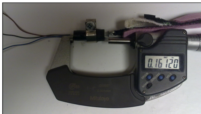
FIGURE 2.12: Respiratory sensor with displacement measured by the micrometer. The internal axis is displaced 0.16120 inches (4.0mm)
