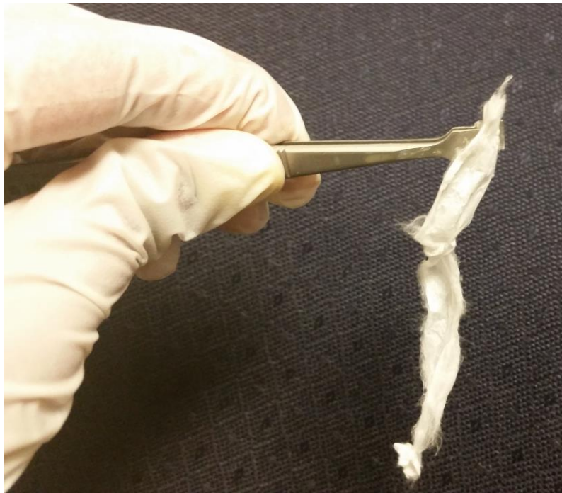
Figure 26: Free standing CoO- ATO nanofibers made with 20% PS in PS: D-limonene
