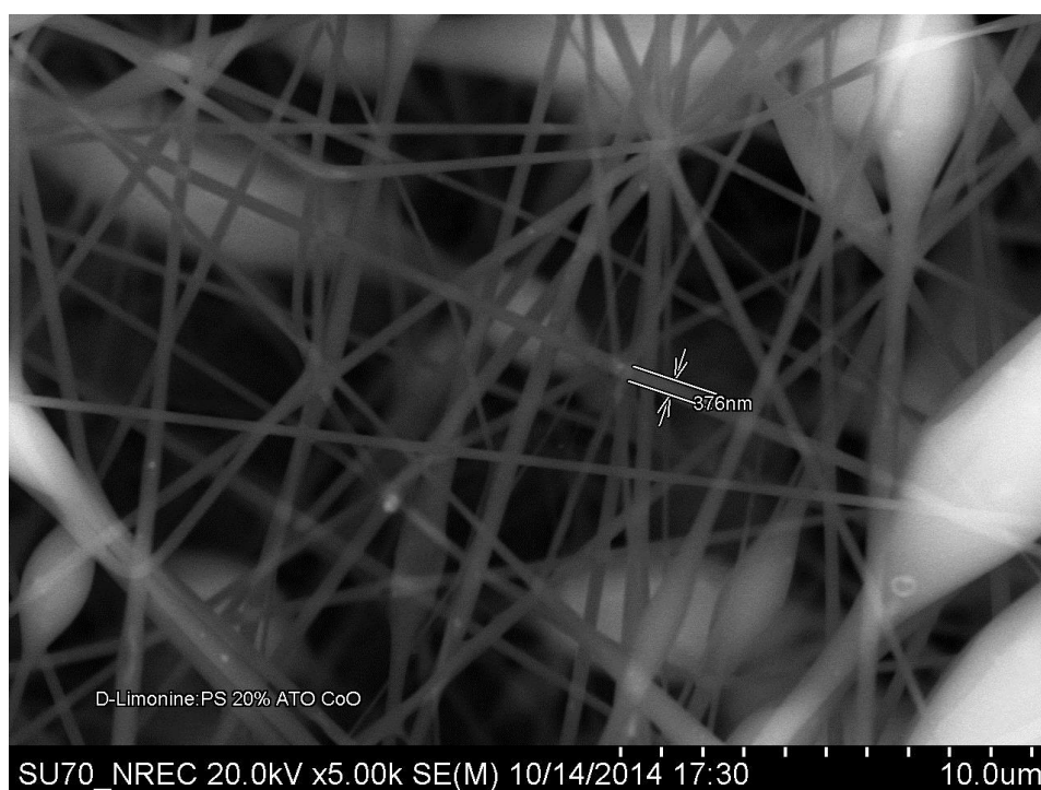
Figure 20: SEM picture of PS: 20% CoO: 10% D-limonene/ATO: 70%
