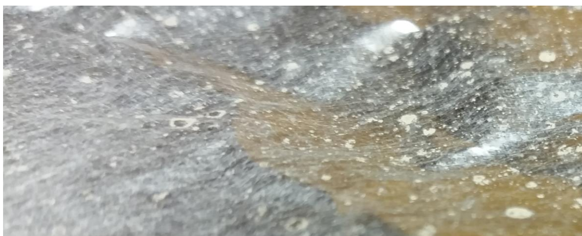
Figure 28: Electrospinning 15% PS in PS: toluene solution with very less distance
