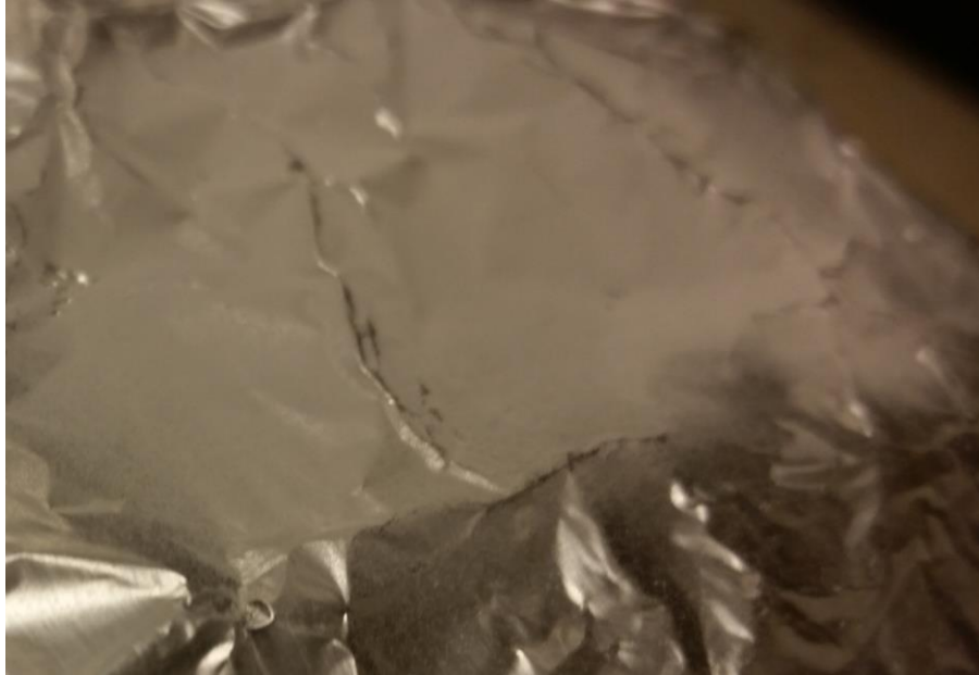
Figure 25: Nanofiber mesh - PS: toluene solution with 20% PS.
