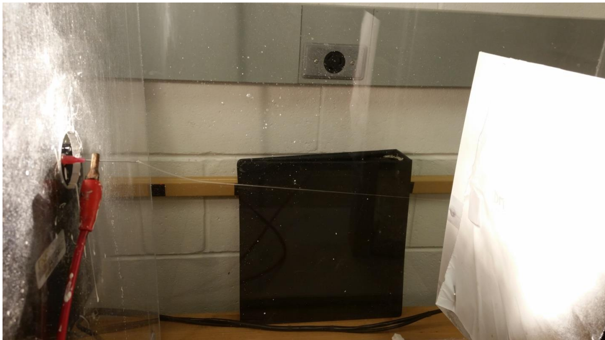
Figure 7: Electrospinning system with a thick bundle of PS fibers
