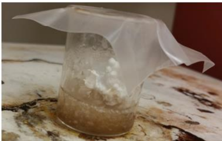
Figure 4: Mixing of CoO-ATO PS: toluene solution on a magnetic stirring plate
