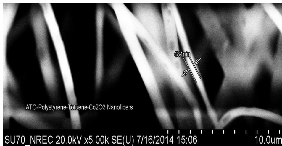
Figure 19: SEM picture of PS: 20% CoO: 10% toluene/ATO: 70%
