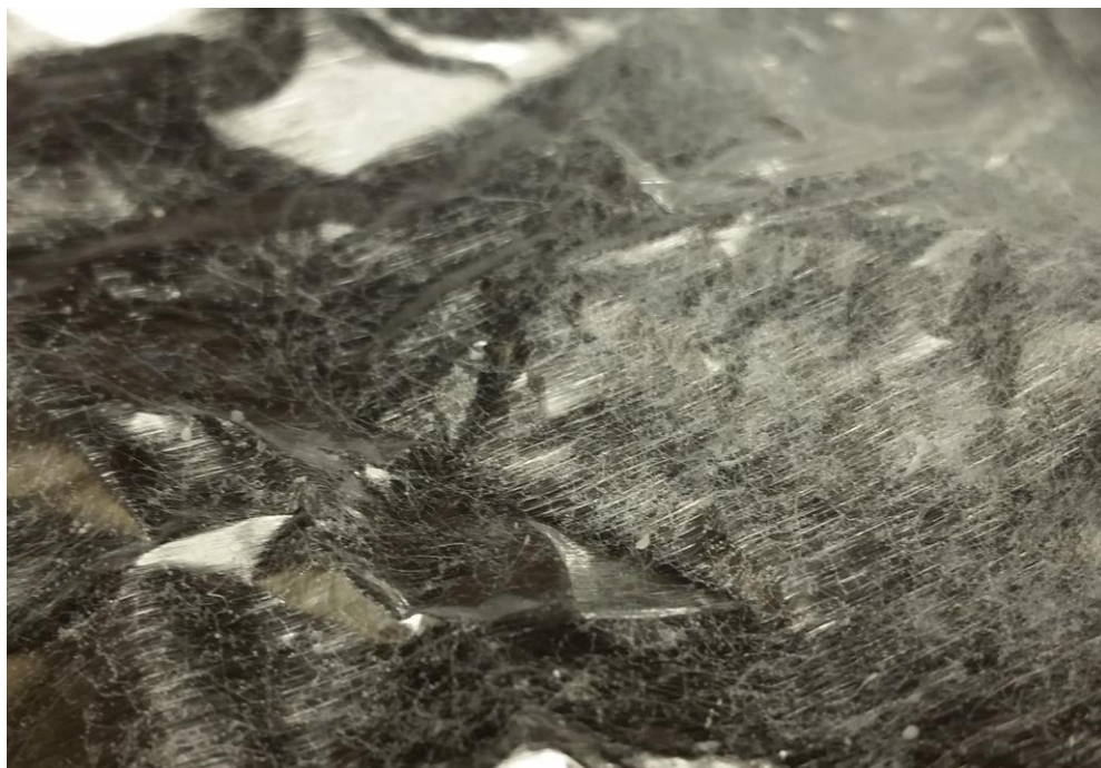
Figure 24: Nanofiber mesh - PS: toluene solution with 10% PS.
