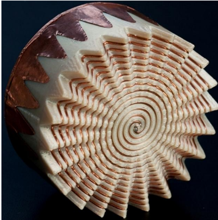
Figure 4.20: Fabricated model of sinuous cavity backed PSA antenna utilizing an exponential growth factor of 3
