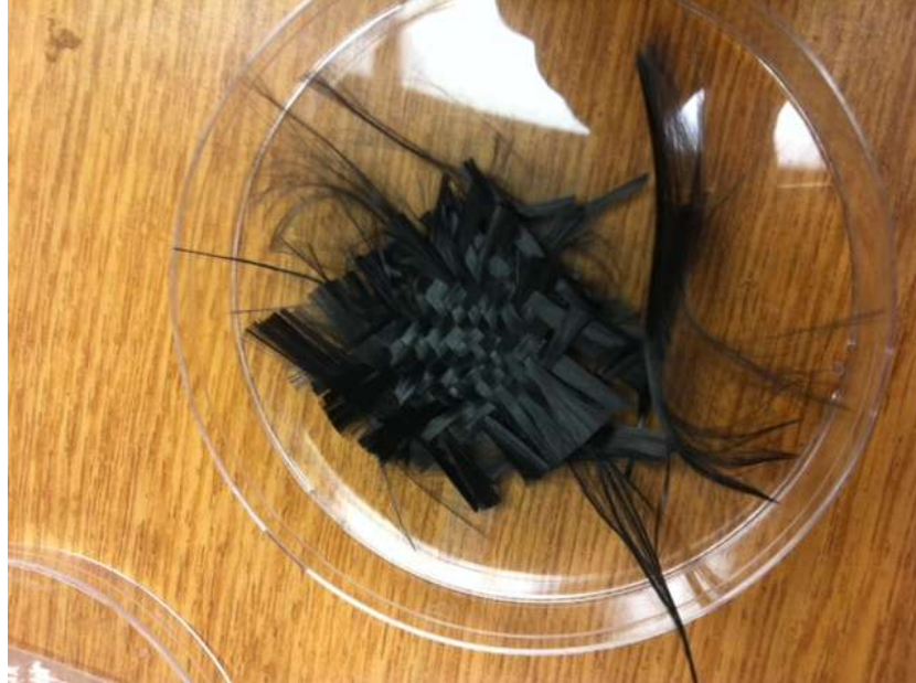
Figure 5.2.2. Piece of interweaved 0°/90° carbon fiber mat.
