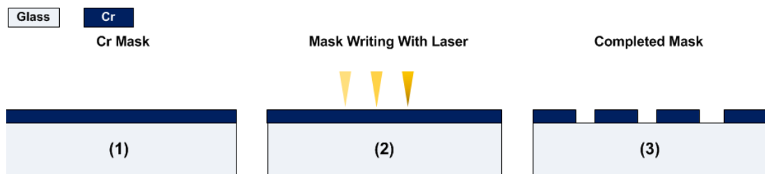
FIGURE 4.3: Process step for mask fabrication from laser ablation system.
