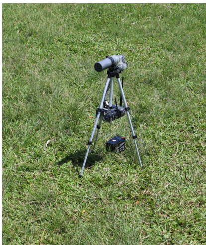
Fig. 3. Snap of complete sensor unit deployed in the field. The microphone and the transmitter units are mounted on a tripod and units are protected with weather shields. Four sets of similar sensor units are deployed for the experiment. The transmitter units were powered by 12 V DC battery.
