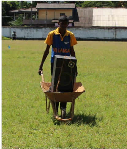
Fig. 5. Picture of the surrogate elephant which is being moved by one of the assistants. The unit consists of sound player connected to a speaker through an amplifier. The system was designed to play previously recorded elephant rumble signals during the experiment.
