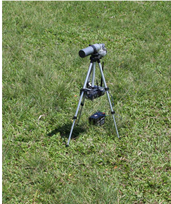
Figure 7.4: Snap of complete sensor unit deployed in the field. The microphone and the transmitter units are mounted on a tripod and units are protected with weather shields. Four sets of similar sensor units are deployed for the experiment. The transmitter units were powered by 12 V DC battery.
