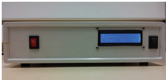
(b) Integrated 16 x 2 LCD unit displaying initialization of the recorder system.
