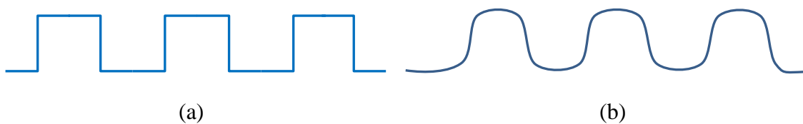
Fig.4. 15: Grating shape: (a) ideal rectangular; (b) practical
