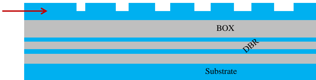
Fig.3. 11: Schematic of the reference grating coupler
