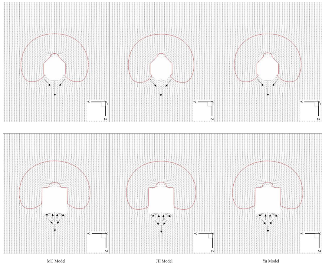
Fig. 4.10 Droplet dynamics as the wetting droplet ( \theta = 62^\circ ) impacts the obstacles for the different pseudo-potential based wetting models at lattice time = 800. The figure shows the interface profile and the velocity vector in the plane x=40 . Arrows are included to show the general direction of the velocity vectors
