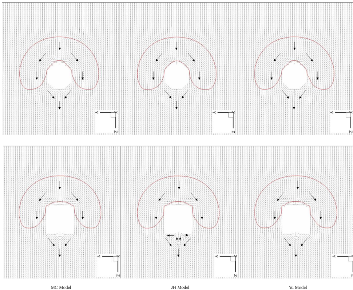
Fig. 4.16 Droplet dynamics as the non-wetting droplet ( \theta = 118^\circ ) impacts the obstacles for the different pseudo-potential based wetting models at lattice time = 800. The figure shows the interface profile and the velocity vector in the plane x=40 . Arrows are included to show the general direction of the velocity vectors.
