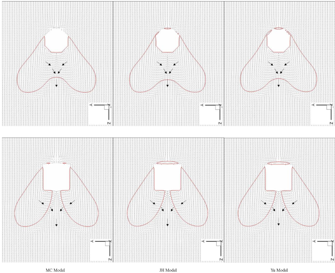
Fig. 4.11 Droplet dynamics as the wetting droplet ( \theta = 62^\circ ) impacts the obstacles for the different pseudo-potential based wetting models at lattice time = 1000. The figure shows the interface profile and the velocity vector in the plane x=40 . Arrows are included to show the general direction of the velocity vectors
