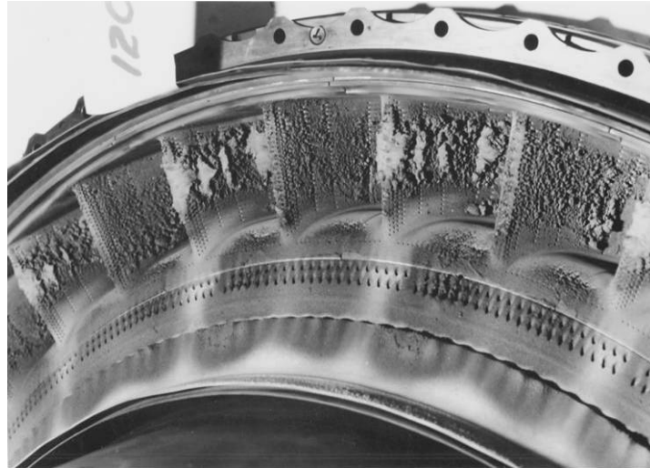
Figure 1-2: Volcanic ash deposition on turbine vanes (Courtesy of A. Hamed et al. [3] )
