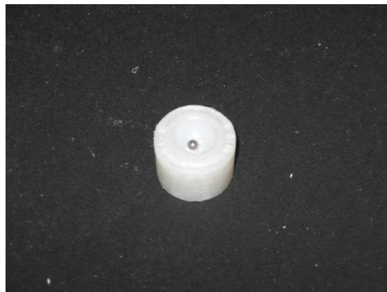
Figure 4-16 Sabot view with launched stainless steel sphere
