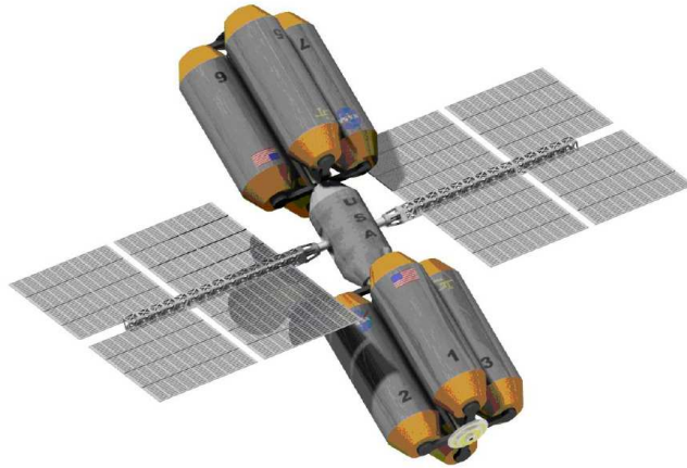
Figure 7: Propellant Depot Concept Art from Georgia Tech Revolutionary Technical Challenge Graduate Research Team, reproduced from [26]
