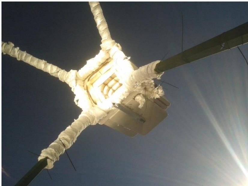
**Figure 5.25 A bottom view of the solar receiver and its support structure during receiver testing with the blue sky in the background.**
