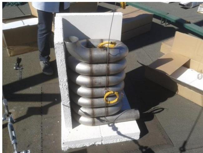
**Figure 5.9 The solar receiver positioned on the bottom insulation before being installed on the receiver structure.**
