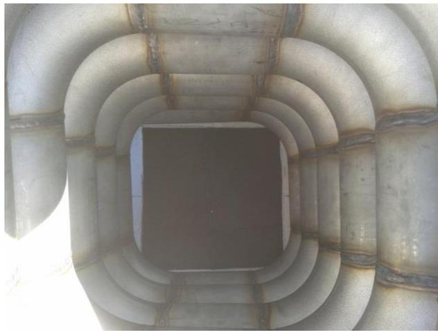
**Figure 5.10 Top view of the solar receiver with the aperture shown at the bottom.**
