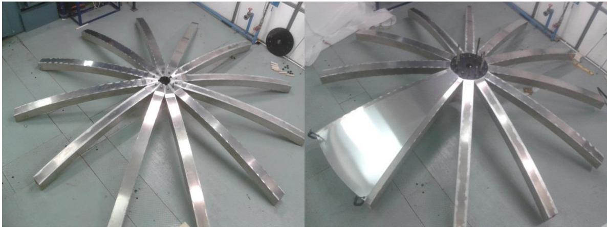
**Figure 5.2 Assembly of the 4.8 m diameter parabolic solar dish in the laboratory (upside down).**
