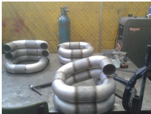
**Figure 5.7 Manufacturing of the solar receiver.**
