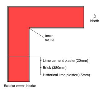
Figure 7-1 Schematic drawing of the base wall corner
