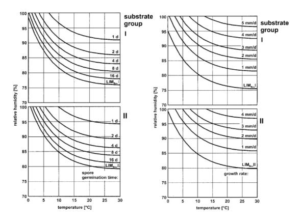
Figure 6-3 Generalized isopleth system for spore germination (left) and mycelia growth (right). Top: isopleth system for substrate category I. Bottom: isopleth system for substrate category II (Sedlbauer 2001)
