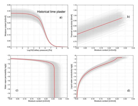
Figure 7-10 Material functions of historical lime plaster a) moisture retention curve b) thermal conductivity c) water vapor permeability d) liquid water conductivity
