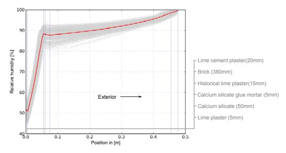
Figure 7-14 Relative humidity profiles in the retrofitted wall in the 175<sup>th</sup> day simulation
