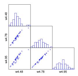
Figure 4-17 Scatterplot matrix of moisture contents w4.48, w4.78 and w4.95 in the plaster/mortar category
