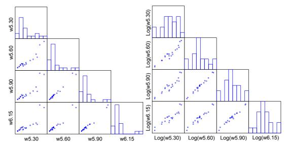
Figure 4-9 Scatterplot matrixes of moisture contents w5.30, w5.60, and w5.90 without transformation (left) and with logarithmic transformation (right) in the building brick category
