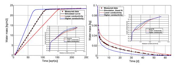
Figure 3-20 Adjustment of liquid water conductivity to match the measured water absorption and drying courses
