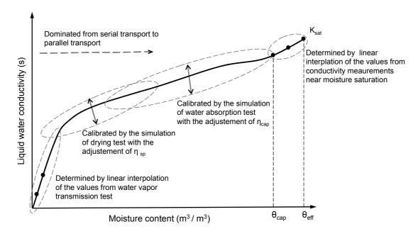
Figure 3-18 Liquid water conductivity function derived from different experiments according to Scheffler (2008)
