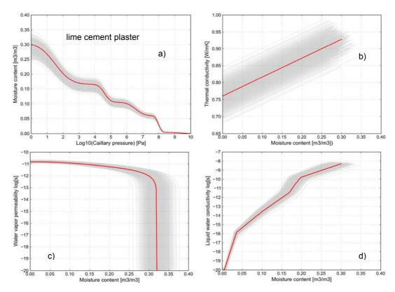
Figure 7-8 Material functions of lime cement plaster a) moisture retention curve b) thermal conductivity c) water vapor permeability d) liquid water conductivity
