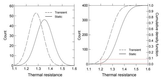
Figure 7-20 Probability density functions and cumulative density functions of transient and static thermal resistances
