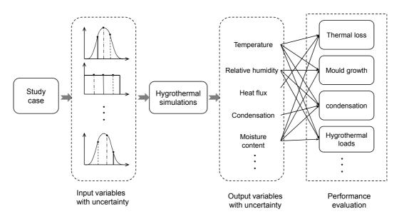
Figure 6-1 Schematic drawing of the probabilistic performance evaluation procedure
