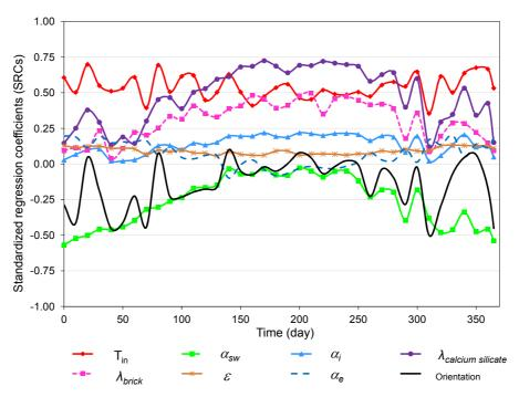
Figure 7-27 PCCs (top) and SRCs (bottom) of the eight influential variables against daily average heat flux through interior surface
