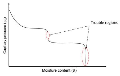
Figure 2-7 Spline interpolation between the measured moisture contents yielding numerical problem
