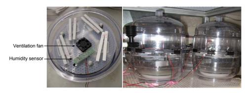
Figure 3-4 Desiccator chambers with the saturated salt-in-water solution
