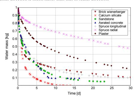
Figure 3-13 Drying behaviors of various building materials
