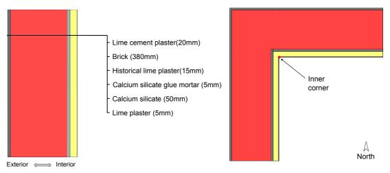
Figure 7-5 Schematic drawing of the retrofitted wall and the corresponding corner
