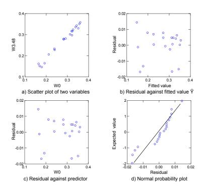
Figure 4-12 Scatter plot of moisture contents w0 and w3.48 and corresponding residual diagnostic plots
