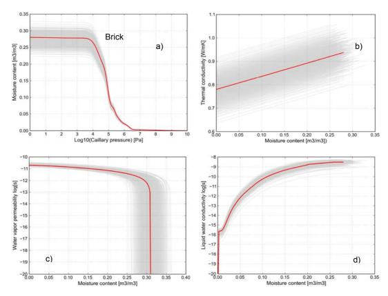
Figure 7-9 Material functions of brick a) moisture retention curve b) thermal conductivity c) water vapor permeability d) liquid water conductivity
