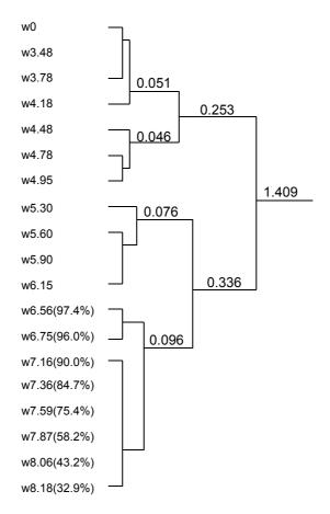
Figure 4-5 Tree diagram of clustering of moisture storage data in the building brick category by using Ward's method
