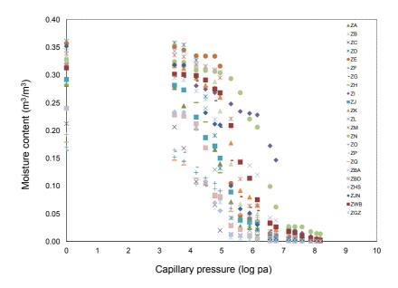
Figure 4-23 Scatter plot of measured moisture storage data of 23 specific bricks
