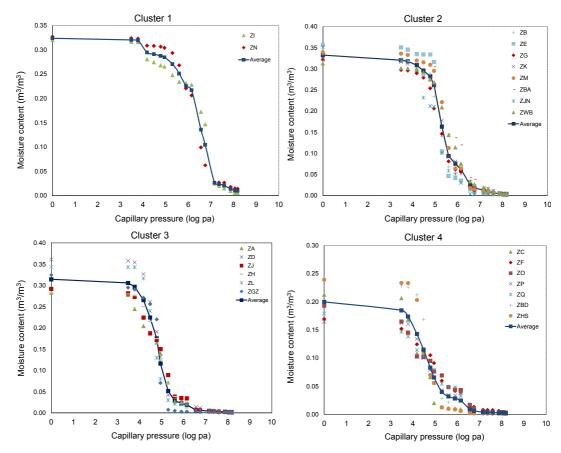
Figure 4-25 Measured moisture storage data and their means in each cluster
