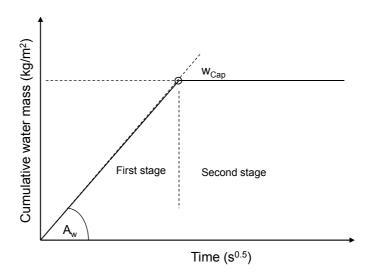
Figure 3-9 Schematic view of one-dimensional water absorption process
