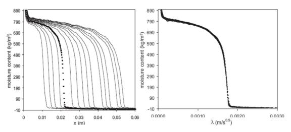
Figure 2-4 Moisture content profiles in the calcium silicate plate subjected to water absorption test (left) and the corresponding Boltzmann transformed data (right) (Carmeliet 2004)
