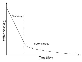
Figure 3-12 Schematic drawing of the drying process
