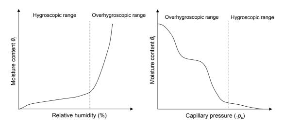
Figure 2-3 Moisture content as a function of relative humidity (left) and capillary pressure (right)
