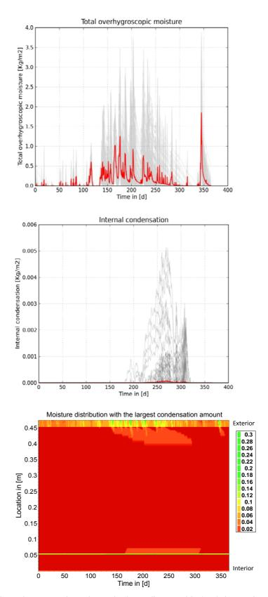
Figure 7-15 Total overhygroscopic moisture in the wall assembly (top), internal condensation (middle), and moisture distribution with the largest condensation across the wall assembly (bottom)
