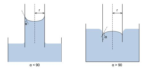
Figure 2-2 Schematic drawing of capillary phenomena in cylindrical capillaries
