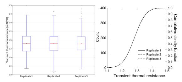
Figure 7-23 Box plot of transient thermal resistances of the three replicates (left) and the plot of their cumulative density functions (right)
