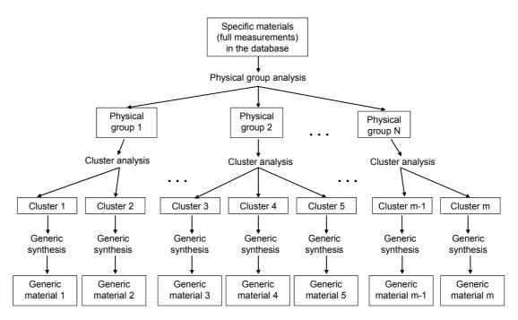
Figure 4-1 Schematic drawing of a systematic procedure to derive generic materials
