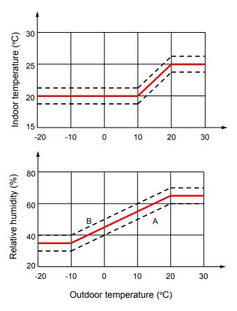
Figure 7-6 Indoor relative humidity (top) and temperature (bottom) function profiles. The dash lines outline the relevant variation range
