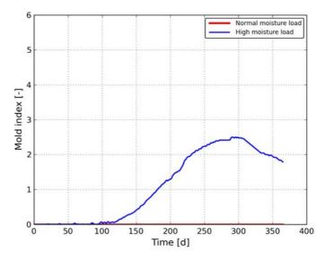
Figure 7-4 Mold index for assessing the mold growth risk at the interior surface of the base wall corner
