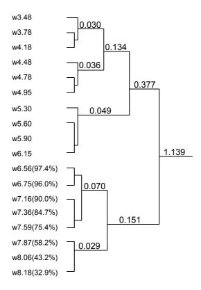
Figure 4-15 Tree diagram of clustering of moisture storage data in the plaster/mortar category by using Ward's method
