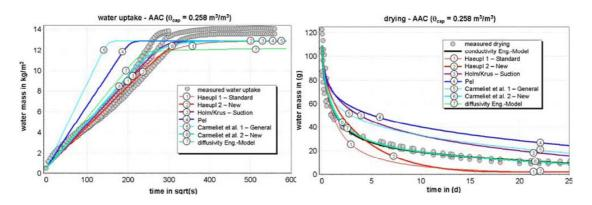
Figure 2-6 Comparison of measured and calculated water absorption (left) and drying (right) behaviors by different diffusivity functions for aerated concrete (Scheffler et al. 2007)
