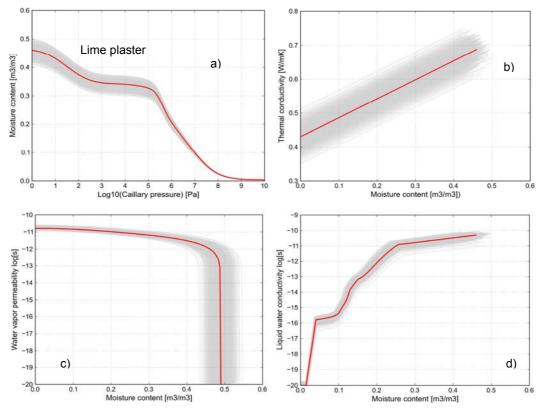
Figure 7-13 Material functions of lime plaster a) moisture retention curve b) thermal conductivity c) water vapor permeability d) liquid water conductivity
