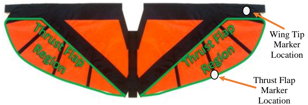
Figure 67. Wing planform showing the thrust flap region and the locations of the wing tip and thrust flap markers.
