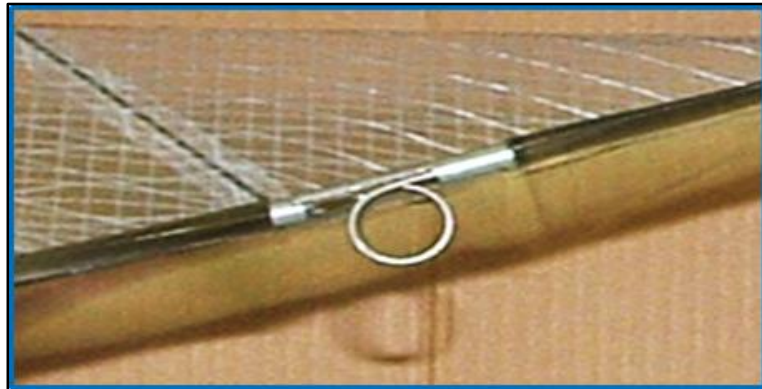
Figure 5. Passive torsional spring that allow for bending only during the upstroke and locks during the downstroke [28].
