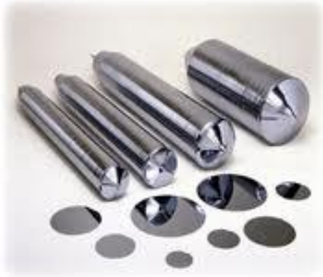
Fig. 2.12. A typical silicon ingot grown using Czochralski method of various wafer sizes. [10]
