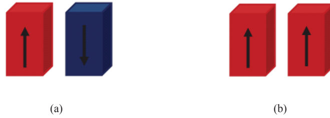
Figure 2.9 (a) Definition of logic '1' and '0' for nanomagnets and (b) Metastable states for coupled pairs.
