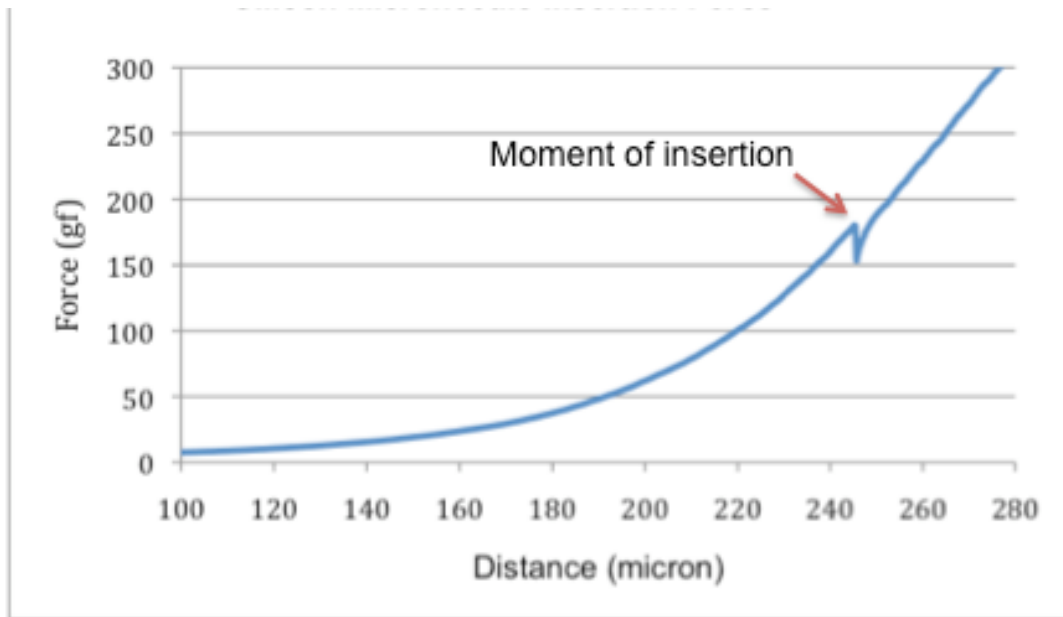
Figure 28: Insertion force of silicon microneedles
