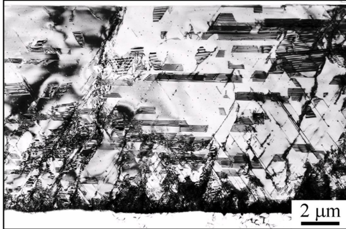
Figure 2.6 Example of hetero defects in (100)3C-SiC from X-TEM. Note the defects along the (111) planes, also threading dislocations and stacking faults. Image courtesy C. Bongiorno, IMM-CNR, Catania, Italy.
