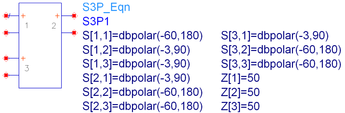
Figure 4-2 EQUATION BASED WILKINSON POWER DIVIDER MODEL An Equation based, ideal Wilkinson power divider represented in Agilent’s Advanced Design System. ‘dbpolar(m,n)’ converts an input of decibels (m) and degrees (n) into a complex value.
