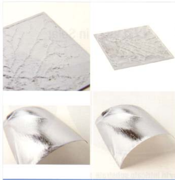
Figure 63. ‘Stress-induced lift-off method’ (SLIM-Cut) process. A high thermal stress is induced by a metallization layer, resulting in the release of a 50 \mu\text{m} Si foil. The top row shows the remaining substrate and the bottom row, the thin lifted-off silicon layer. [84]
