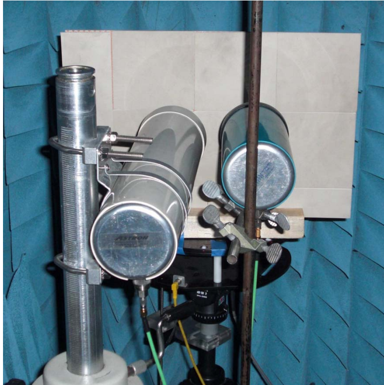
Figure 5.17 – Measurement on covered JC-FSS.
