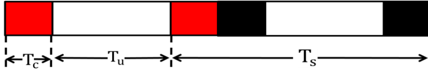
Fig 4.7 The structure of the OFDM symbols
