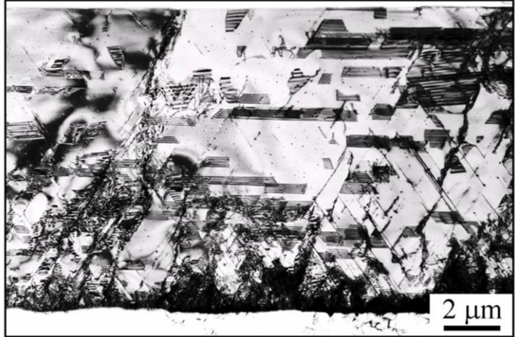
Figure 2.8 Example of hetero-defects in (100)3C-SiC from X-TEM. Note the defects along the (111) planes, also threading dislocations and stacking faults. Image courtesy C. Buongiorno, IMM-CNR, Catania, Sicily (IT)
