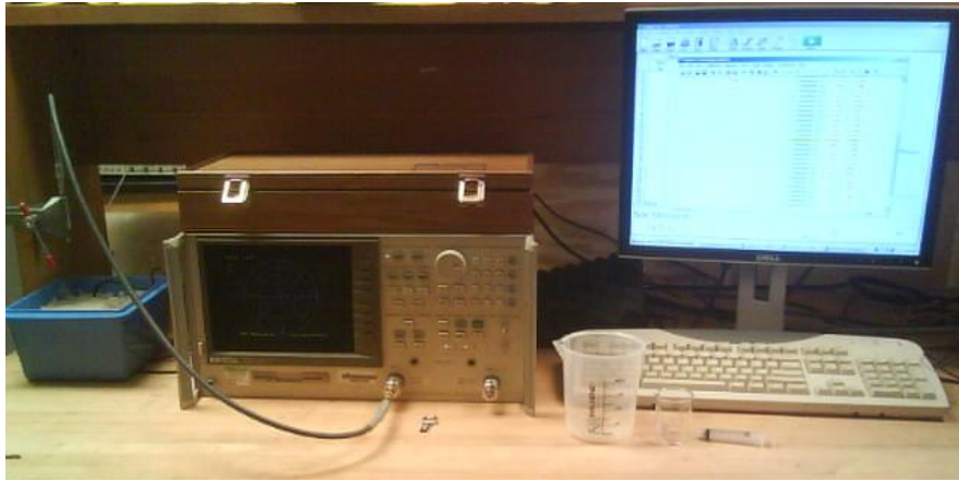
Figure 2.6 Measurement setup for permittivity measurement.
