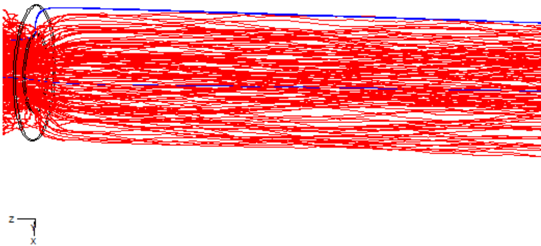
Figure A.6: Particle traces near orifice; Red = injection particle, Blue = trace of pipe walls. r = 2.25 , Re_{main} = 434,856 . Re_{inj} = 299,054 . P = 192.4 kPa.
