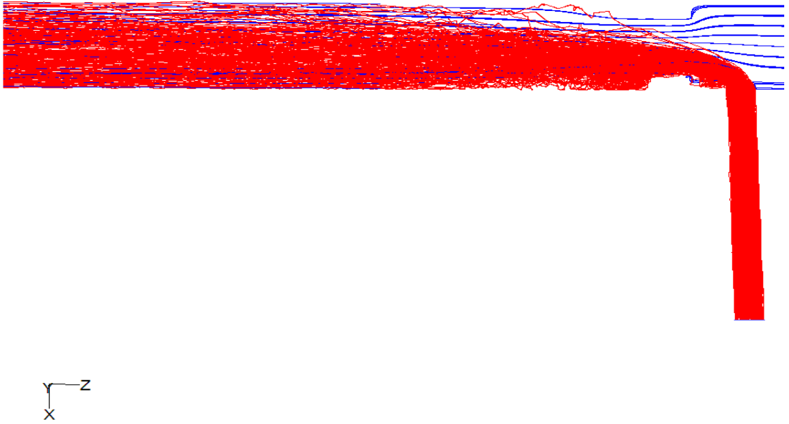
Figure A.18: Particle traces near injection; Red = injection particle, Blue = trace of main flow. r = 1.33 , Re_{main} = 465,297 . Re_{inj} = 176,756 . P = 210 kPa.
