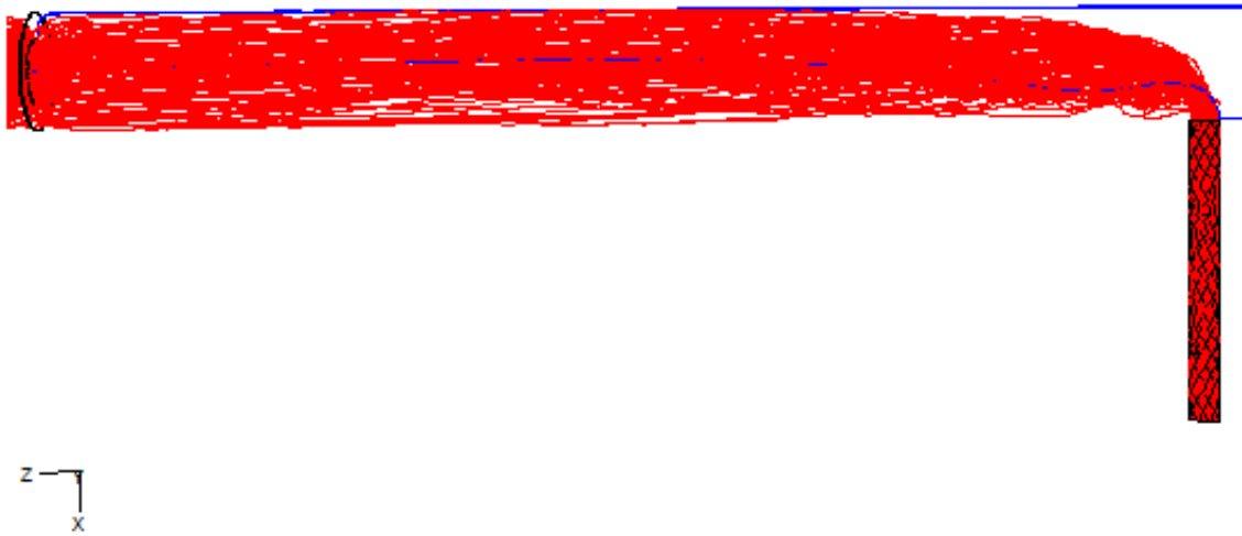
Figure A.5: Particle traces from injection to orifice; Red = injection particle, Blue = trace of pipe walls. r = 2.25 , Re_{main} = 434,856 . Re_{inj} = 299,054 . P = 192.4 kPa.
