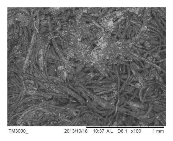
**Figure 2.1**: Woollen fibres matted by fulling as viewed under a scanning electron microscope. This fragment of cloth, attached to a late medieval or early modern lead cloth seal, was retrieved from the River Wear in Durham city.<sup>28</sup>
