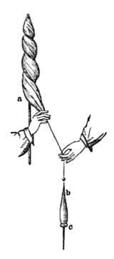
Figure 2.2: Hand or drop spindle with distaff.<sup>33</sup> A. Distaff B. Spindle C. Whorl
