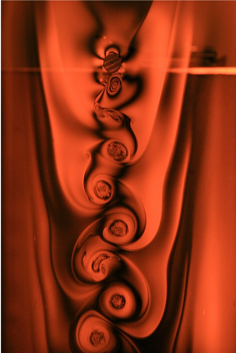
Figure 1: Vortex shedding in a soap film
