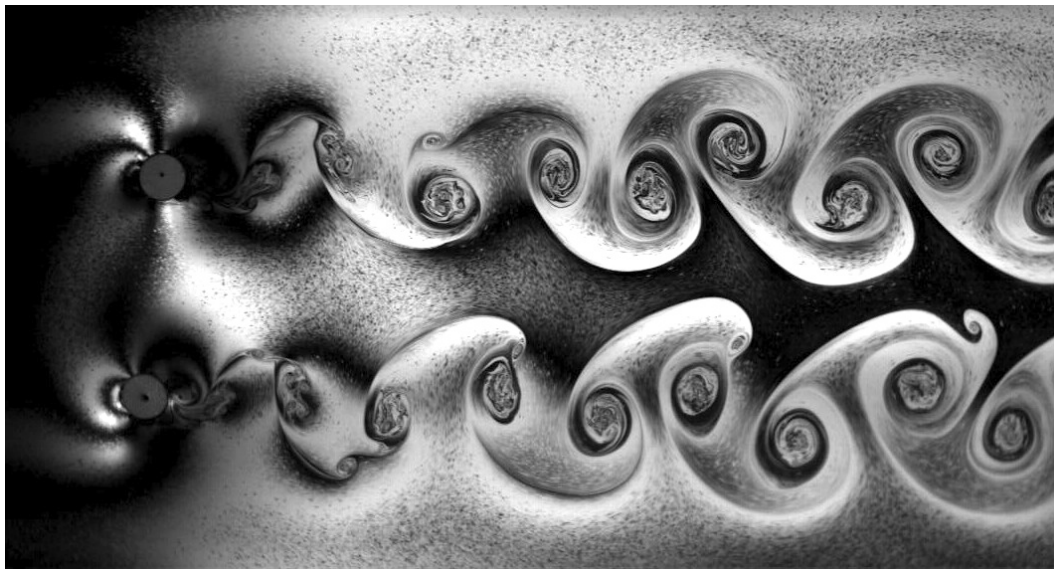
Figure 21: Example of soap film visualization, with two disks side-by-side. Flow is from left to right.
