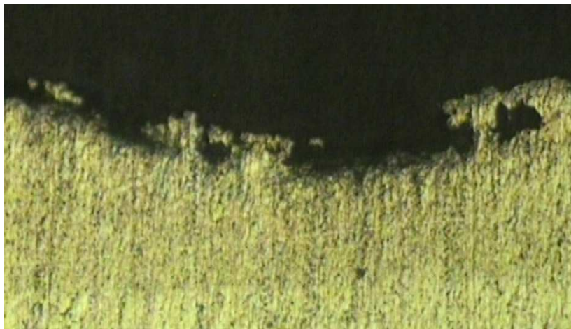
Figure 3.2-4: Impacted surface layer after three electrical arcs (x200)
