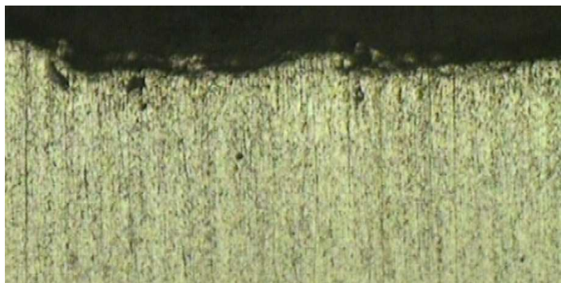
Figure 3.2-2: Section of the anode after one electrical arc (x200)
