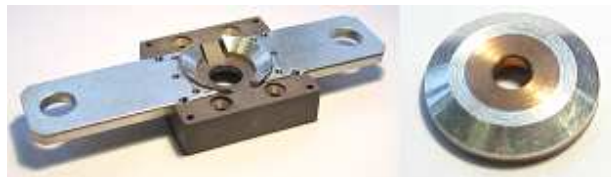
Figure 4.2-1: Pictures of the static and the moving contacts used in this experiment
