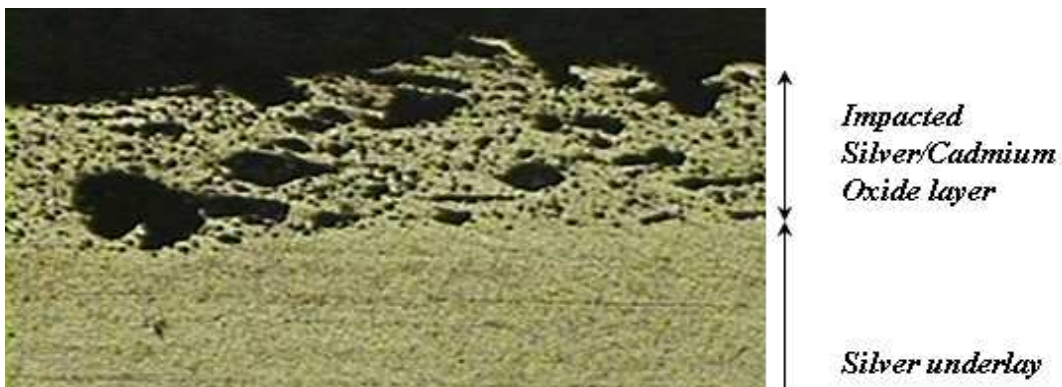
Figure 2.3-2: Section of the anode after one electrical arc (25x)
