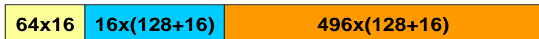
Figure 18. OFDM frame structure in serial representation. The first 1024 samples are for symbol synchronization, followed by 16 pilot symbols for channel estimation and data payload of 496 symbols. Each symbol consists of 144 samples.
