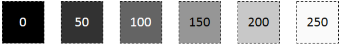
Figure 2.2: Examples of the six unique modulation levels used in testing (with corresponding 8-bit RGB greyscale value).
