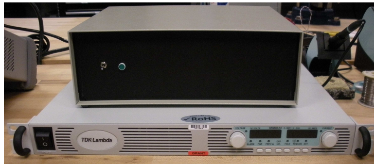
Figure 4.13: Photograph of the Lambda GEN600-2.6 DC Power Supply and the custom electronics box containing the Acopian power supply that are used to power the 600PST SparkJet circuit.
