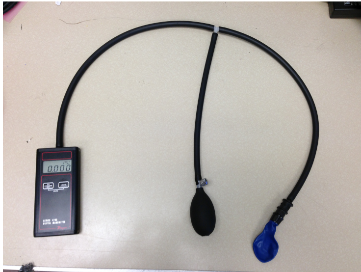
Figure 3.1: Device created to measure the pressure on the eye
