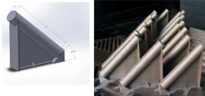
Sample orientation: inclined 45°
