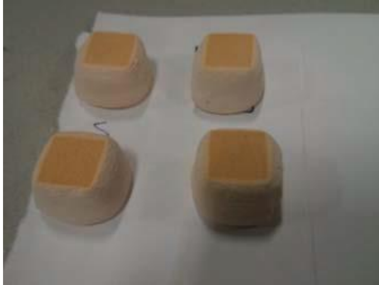
Fig. 2.5 Printed parts after curing [13]
