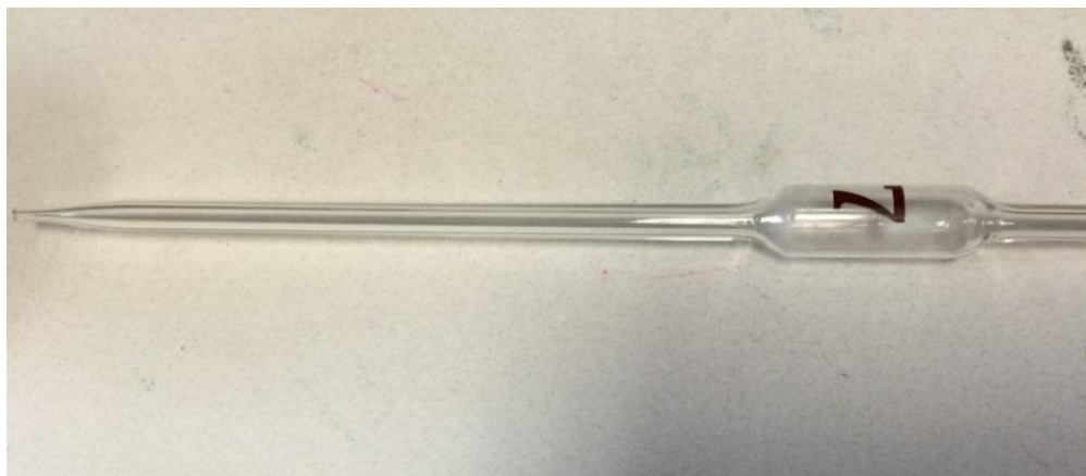
Fig. 7.4 Volumetric pipet used for measuring the surface tension of the binder
