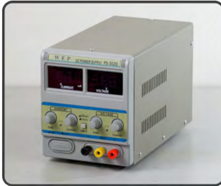
FIGURE 23 - WEP PS-302D DC power supply used to power the rotational motor in Flow Design 2.
