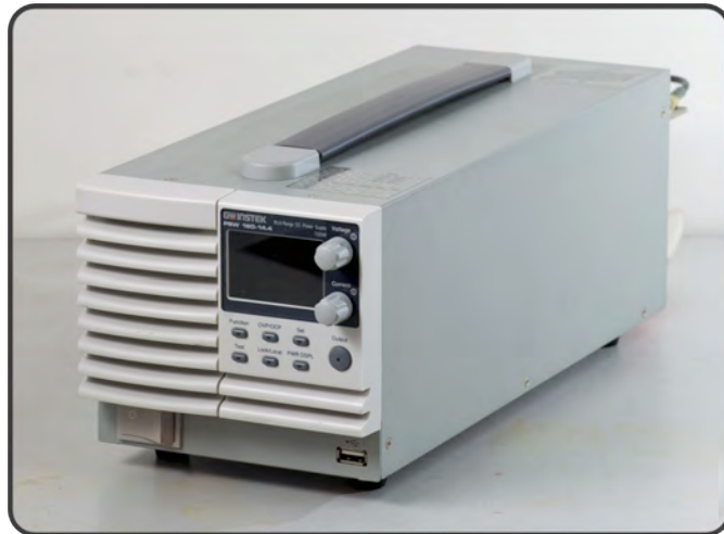
FIGURE 18 - Gwinstek PSW 160-14.4 constant power supply implemented within Flow Designs 1 and 2. Featuring USB and GPIB interface controls, the power supply adds long term functionality, allowing control within LabView. As in this project, the power supply is many times the most costly single component of an electropolishing system.
