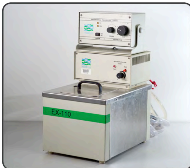
FIGURE 22 - Neslab EX-110 water heating/cooling pump used to control the temperature of the by controlling the temperature of water that was sent through the Flow Design condenser.
