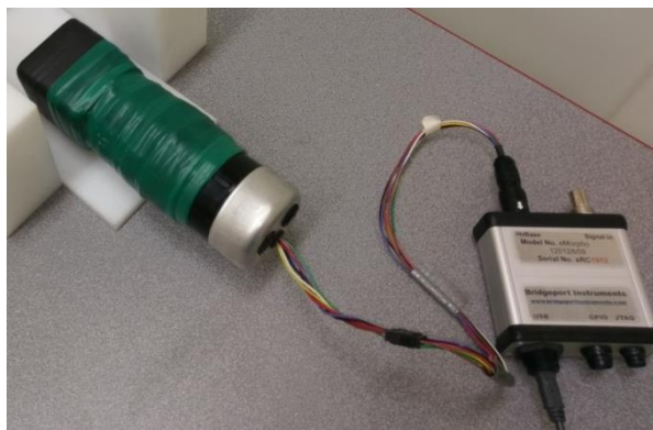
Fig. 57. Detector assembly for PSD testing of EJ-299-33A
