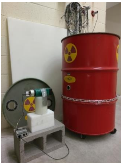
Fig. 58. Detector set-up for PuBe measurements
