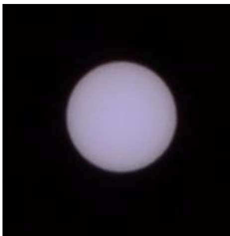
Figure 3. Image of the Sun using 4-ND8 and 1-ND4 Filters
