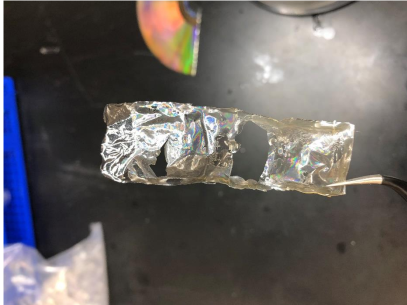
Figure 7: Nanoimprinted silk film with significant dissolved sections.
