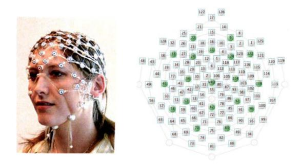
*Figure C1*. (Left) Well placed sensor net and (Right) EGI System for average mastoid reference in International 10-20 montage.
