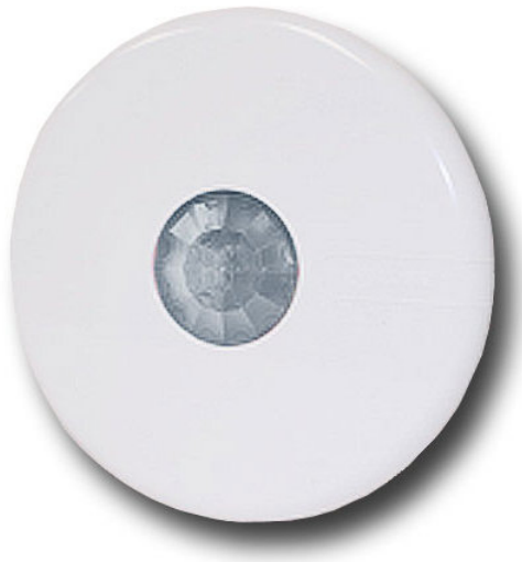
Figure 3.16: Passive Control4 sensors in the second generation sensor network at CASAS. These wireless ZigBee Pro devices (except for 3.13) connect to a permanently powered Control4 device (see Figure 3.17, or 3.13) to transmit sensed events along the mesh to the base station as they can only be leaves in the mesh due to a power saving feature that turns off the radio for minutes at a time.
