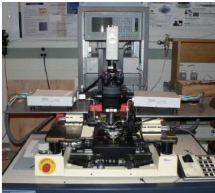
Figure 7.3: Actual Millimeter Wave Test Set-up Used to Measure the MIM Diode
