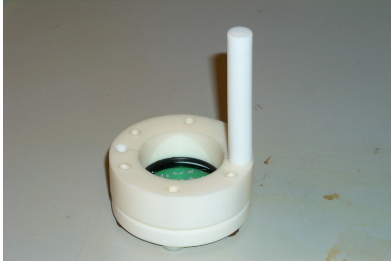
Figure 5.7: Etch Set-up Developed for Silicon Membrane Etching
