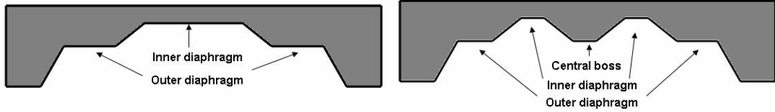
Figure 3.8 Proposed diaphragm architectures a) reinforced diaphragm, b) with bossed structure.
