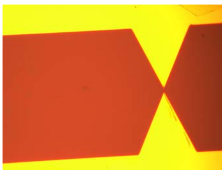
Figure 8.4 Single pair of electrodes for nanowire assembly.
