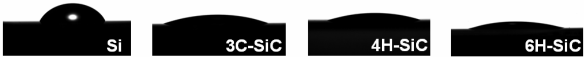
Figure 3.12. Measured water contact angles on Si, 3C-, 4H-, and 6H-SiC surfaces. Note the higher hydrophobicity of Si. In this experiment surface roughness does not influence the contact angle values since all the samples display similar values of R_q .
