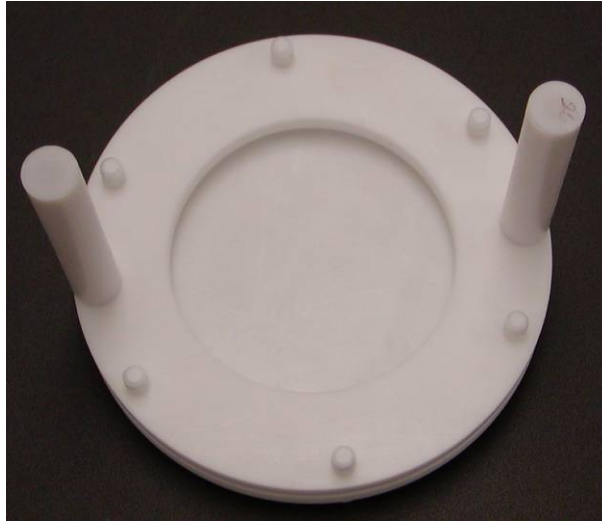
Figure 6.9 100 mm Jig for Backside Wafer Protection During Etching
