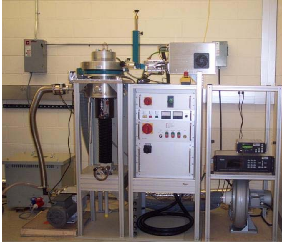
Figure 3.2 Cyrannus I Iplas Microwave Plasma Enhanced Chemical Vapor Deposition System
