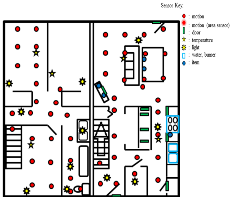
Figure 2.1: The Kyoto smart home testbed floor plan and sensor layout.
