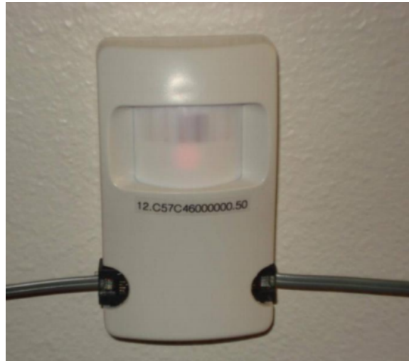
Figure 2.3: Passive infrared motion detector used on CASAS smart home testbeds (adapted from [36]).
