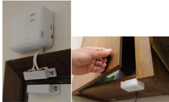
Figure 2.4: Magnetic door sensors on the door (left) and cupboard (right) (adapted from [36]).
